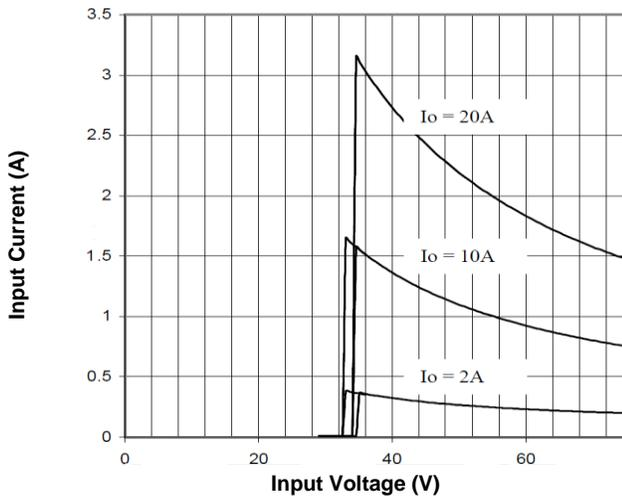
**Figure 9. Input Characteristics**
