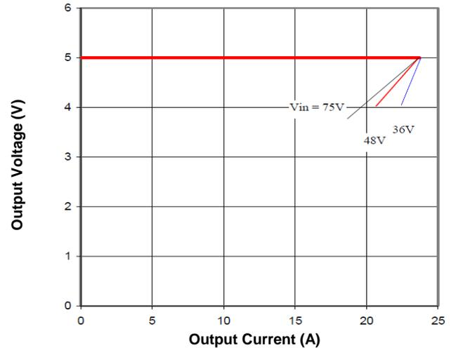
**Figure 10. Output Characteristics**
