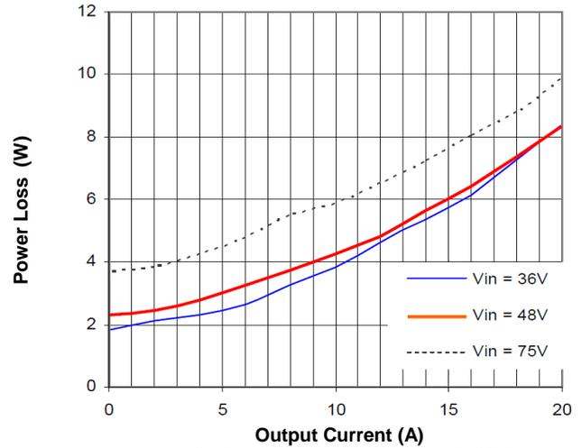
**Figure 2.** Power Loss vs. Load Current (25°C)
