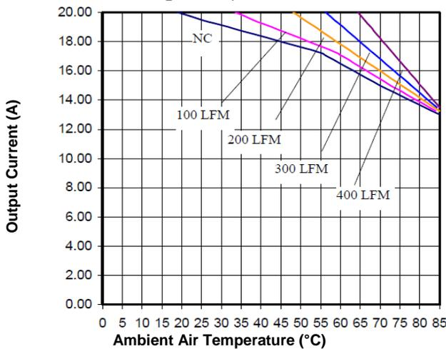
**Figure 11. Current Derating Curve for Airflow Direction 3**
