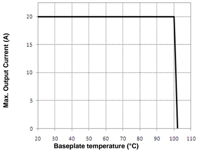
**Figure 13.** Current Derating Curve for Baseplate
