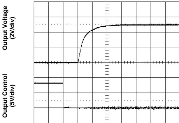
**Figure 3.** Start-Up from Enable Control
