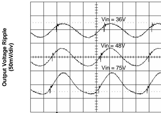
**Figure 5.** Output Ripple Voltage at Full Load
