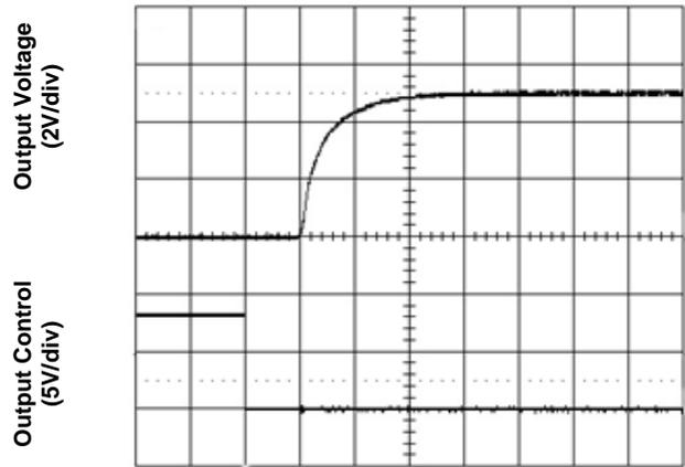
**Figure 4.** Start-Up from Enable Control
